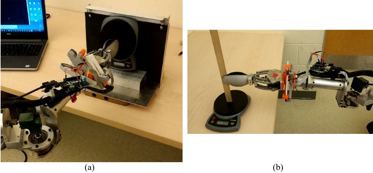
Figure 8.4: (a) test setup 1 using force measurement axis and (b) test setup 2 using moment axis of sensor.
